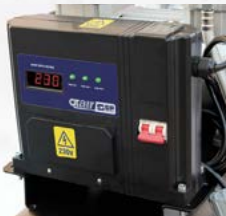
MAINS SUPPLY CONTROL BOX INITIATES START-UP FROM 16A SINGLE PHASE SUPPLY
